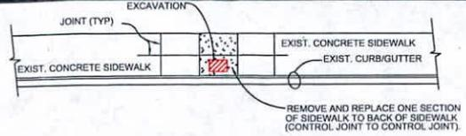
**SIDEWALK REPAIR DETAIL**
